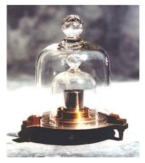
K48 [here to the left] came from the second batch of kilogram replicas to be produced. It was delivered to Denmark in 1949 with an official mass of 1 kg+81 µg. Like all other replicas, it is stored under two nested bell jars virtually all the time. Still, its mass and that of the IPK diverged markedly in only 40 years; the mass of K48 was certified as 1 kg+112 µg during the 1988–1992 periodic verification.
